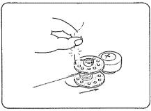
bobbin onto bobbin winder Wind thread until winder stops. Remove spindle with end of thread coming from the top of the bobbin. Push bobbin winder shaft to the right until it clicks. Holding onto end of thread, start machine. When bobbin is slightly filled, snip off end of thread.
